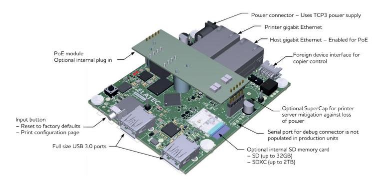
×From secure printing to industrial robotics, TCP3 enables user authentication and access control security for devices that lack a USB port.
